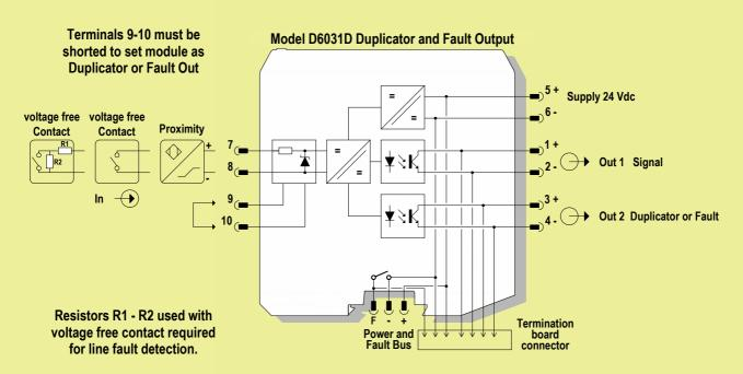
Internal Dip switches programmable
